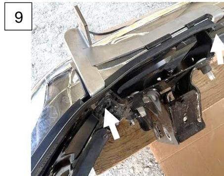
10. With a razor knife, trim the weather seal along the dotted line as shown to allow space for the bracket. Install the weather seal fasteners. Push the bracket down against the bumper and tighten the bolts with the 13mm socket. Repeat steps 9-10 for the opposite side. Reinstall the bumper back onto the vehicle by following steps 2-7 in reverse.
