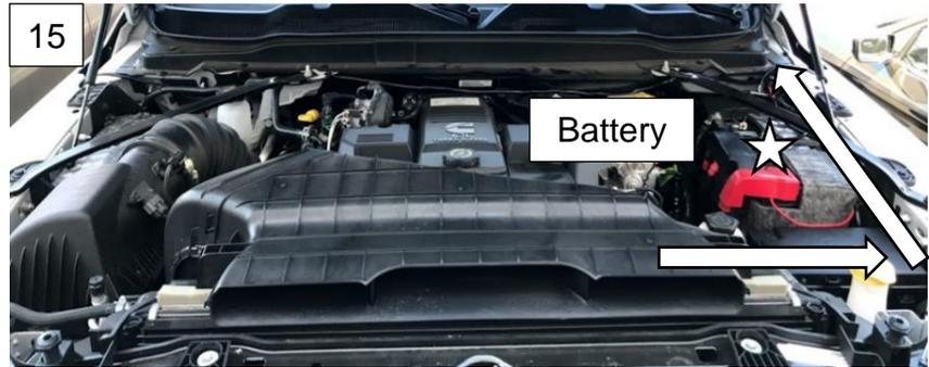
15. Following the path shown, attach the battery leads of the harness to the battery (starred) and mount the relay to a nearby 10mm hex head bolt.
