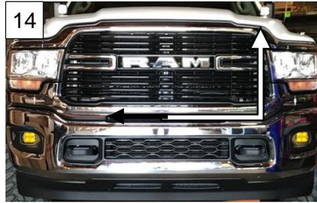
14. Route the light plug end of the harness from the engine bay down to the light following the path shown.
